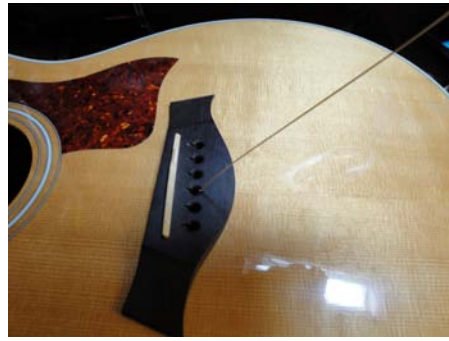
b. Tilt the string away from the neck and aim it at the string slot in the anchor bracket while also pulling up on the string until you feel it “anchor” against the bridge plate.
