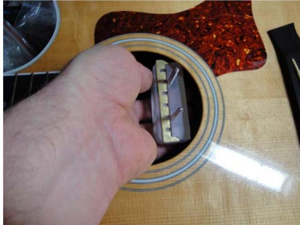
**Insert anchor bracket/tool through soundhole**
