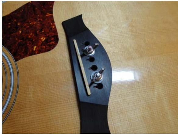
Install the wing nuts on the studs and tighten. After 15 seconds, unscrew wing nuts and remove washers and tool from guitar. Install your strings.
